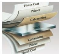
Hot-dipped galvanized steel interior and exterior skins with a baked-on primer and top coat help ensure a virtually maintenance-free door with long-lasting beauty.
